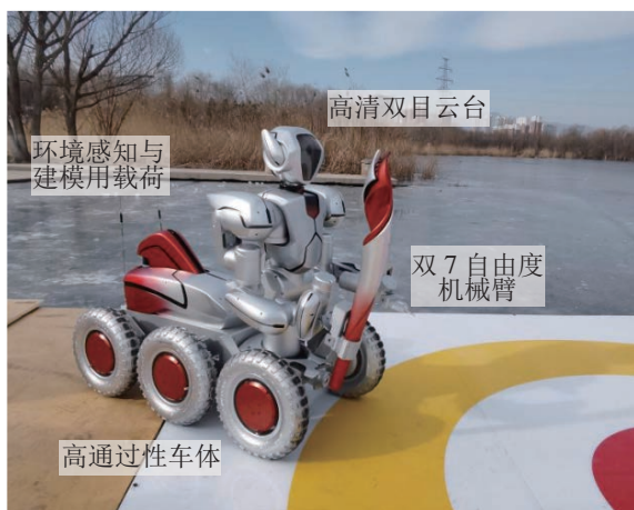
图8 地面机器人及系统组成 Fig.8 UGV and its system composition
